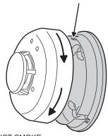
TWIST SMOKE ALARM CLOCKWISE TO LOCK ONTO MOUNTING PLATE
